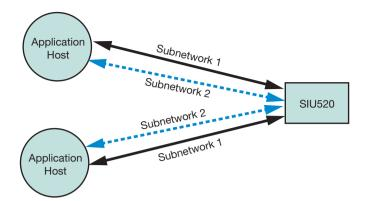
Figure 15. Dual LAN Operation on the SIU520
